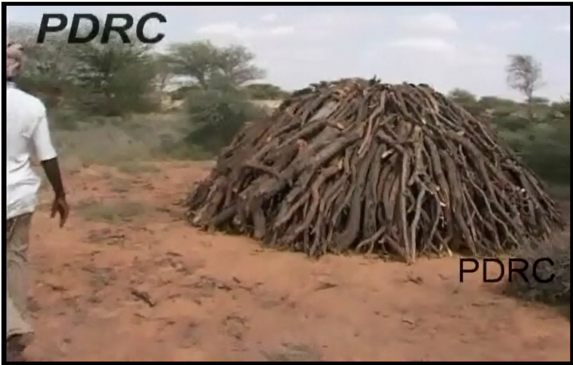
Figure 9 – Timber mound before being buried. Screen shot from a Puntland Development Research Center (PDRC) video.
