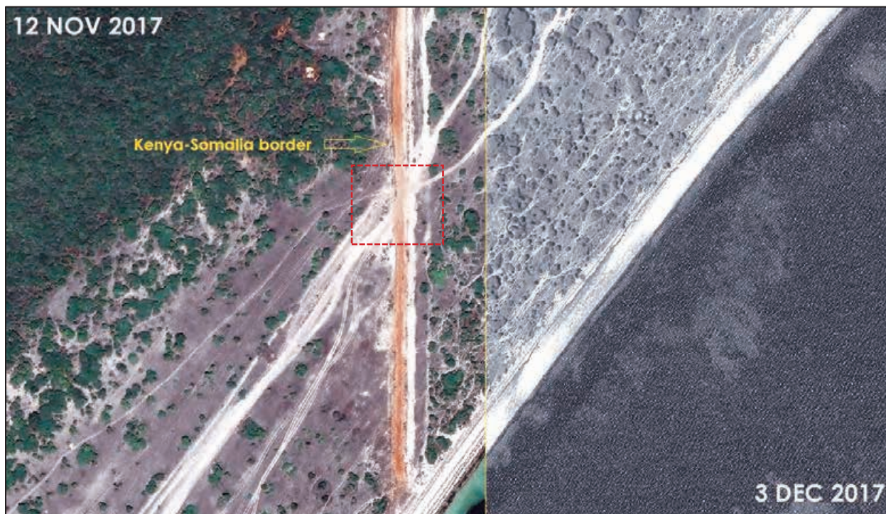
Fig.36 - The figure shows the mosaic of two images taken in the same period (end of 2017) along the Kenya-Somalia border. The red outlined box indicates the point used by trucks to cross the border. Several fresh tracks originating from this point are detected - © [2017] DigitalGlobe
